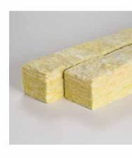
The advanced technology used to manufacture MinWool Safing Insulation ensures consistent product quality, with high fiber density and low shot content, for excellent performance. Safing Insulation is manufactured in a standard 4" thickness. thickness, and is available plain or faced with a (FSP) Scrim Reinforced Foil Facing vapor retarder on one face. It is inorganic and will not mildew or support corrosion.
